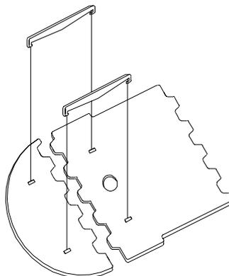
Slide FB-1 and FB-2 together as shown above. Hook the Uplift Connector Bar into the FB-2 floorboard, and use a moderate pressure on the FB-1 to pull it into position so that the Uplift Connector Bar will hold both boards snugly together. Repeat with the other Uplift Connector Bar. Slide the assembled boards into the bow of the boat. The SE290N does not have a FB-2 floorboard and Uplift Connector Bars. Simply insert the FB-1 into the bow of the boat.
