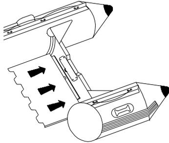
The FB-4 is the rearmost floorboard which has a smooth rear edge and interlocking grooves on the front edge. Place FB-4 at the rear of the hull and slide under the transom lip. Sit in the hull and force the FB-4 under the transom lip with your feet.
