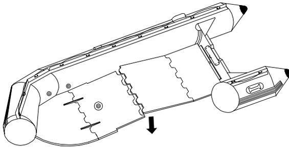
The last floorboard to be inserted is FB-3. Insert FB-3 so it meshes with FB-4 at the stern of the boat and overlaps FB-2 (or, in the case of the SE290N, the FB-1). Lift the ends of FB-2 (or FB-1) and FB-3 and connect the floorboards forming an inverted "V". Step down on the joint. (see above diagram) The boards will snap into place.
